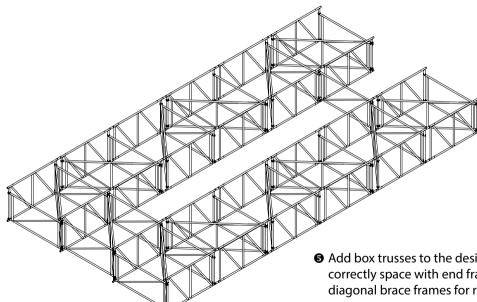
• Add box trusses to the desired width and correctly space with end frames and plan diagonal brace frames for rigidity.
