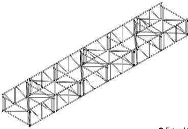
Extend the box truss to the desired length with additional main frames, spigots, end frames and plan diagonal brace frames.
